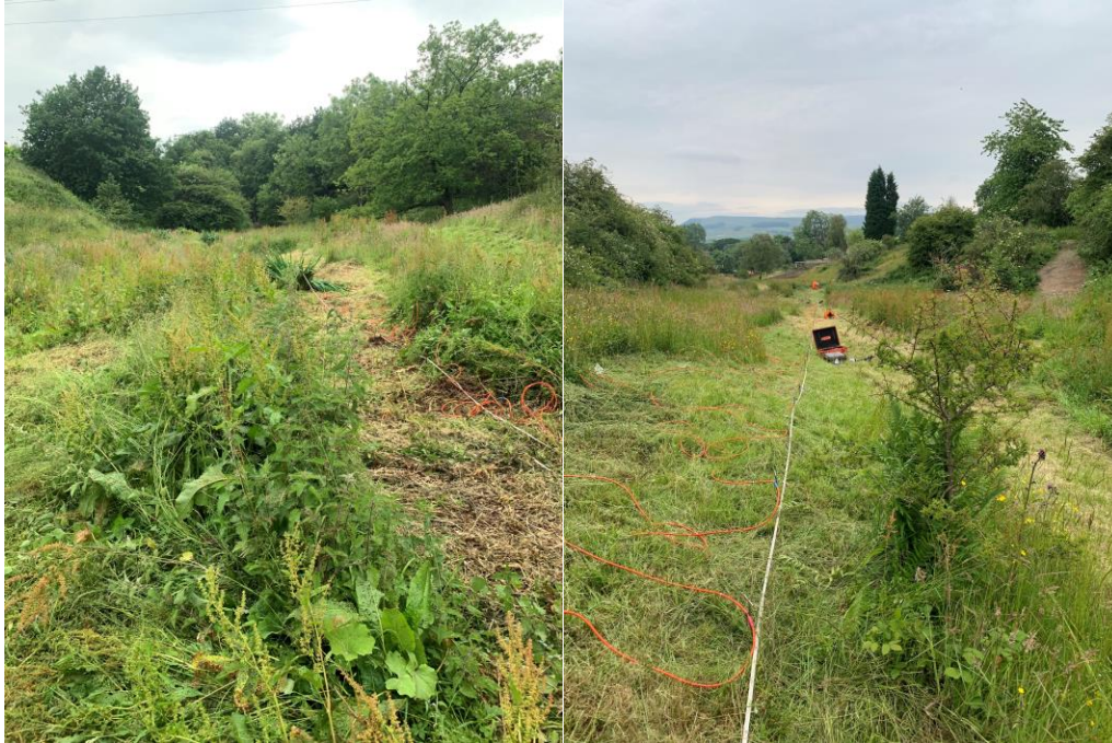
Figure 1: Position of ERT lines across the site.
